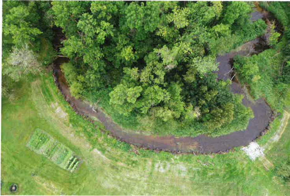
Above: Aerial view of streambank stabilization project completed at the Victor Lundemo and Jason Eichenberger properties utilizing a combination of toe wood (root ball) and rip-rap methods of stabilization.
