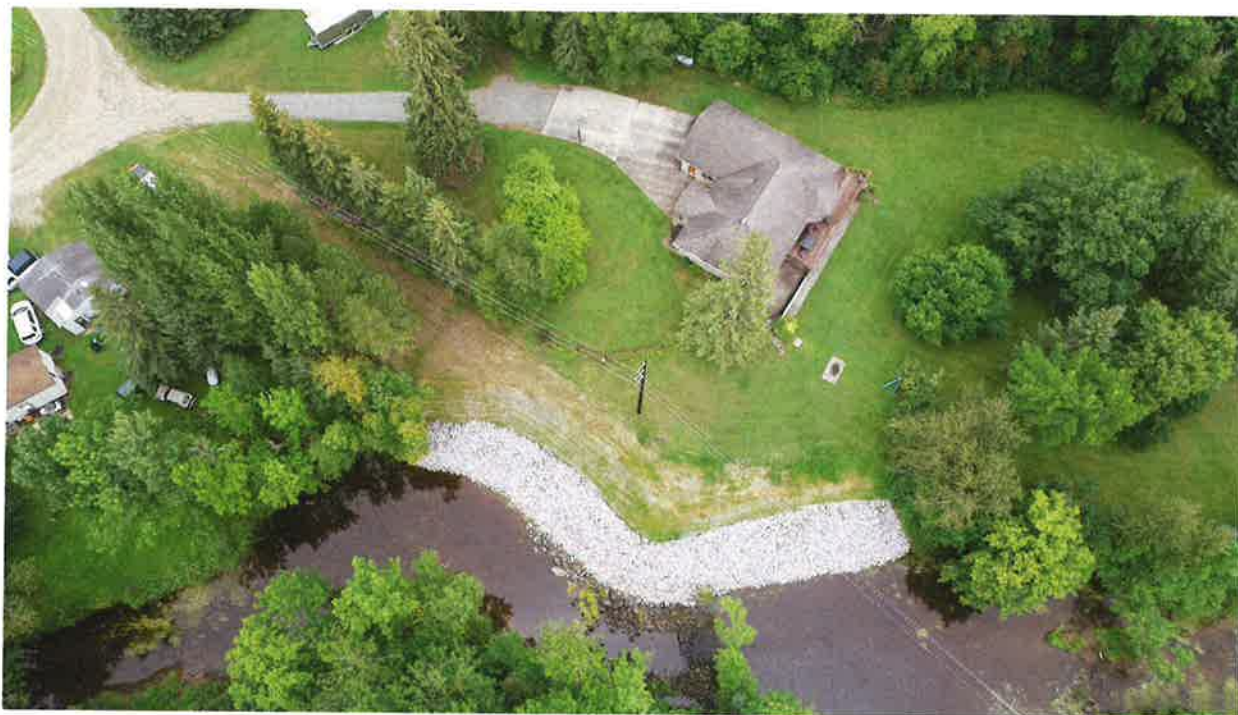
Above: Aerial view of streambank stabilization project completed at the Mike and Carla Roberts properties utilizing rip-rap method of stabilization.
